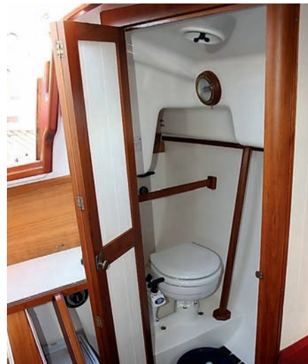
The heads. The space behind the loo is the wet locker and boot rack. Note the grab rail alongside the toilet.
