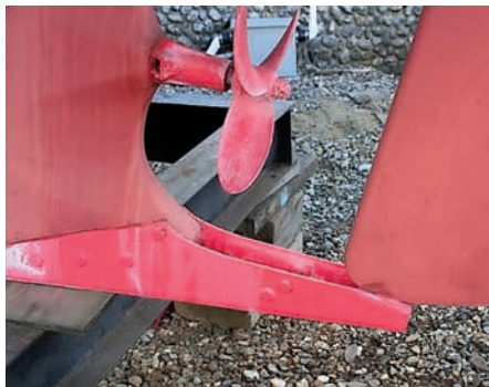
The rudder skeg is made in two sections bolted together. Unbolting the aft end of the skeg without having to remove it completely from the hull makes dropping the rudder easy.
