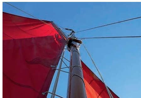
The high peaked gaff's leather-clad jaws swivel round the mast on a strong leather collar.
