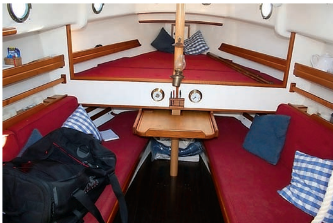
The interior of the Smuggler. The forward berth is raised to provide underneath storage and trotter boxes for the saloon berths. The table is in its stowed position.
