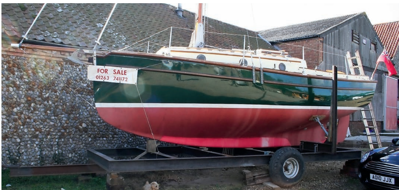
The Smuggler has a sea-kindly hull form. Her shallow draught makes her ideal for creeping up quiet creeks, while the centreplate allows her to go seriously to sea.
