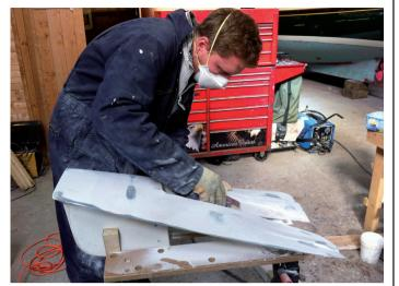
ork has finally begun on the build of the newest addition to the Norfolk Range, 'The Norfolk Explorer'. Chris and Neil are busy making the necessary changes and adjustments to the Oyster hull mould before beginning to create the inner moulding. We anticipate that it should be ready to preview for the Holkham Country Fair.
