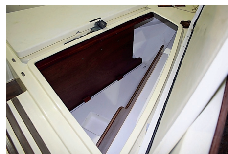
The forepeak is divided into sections. The starboard side has mouldings to support an outboard engine while the port side is used for sails, covers and general gear. Both sides have high-fiddled shelves.
