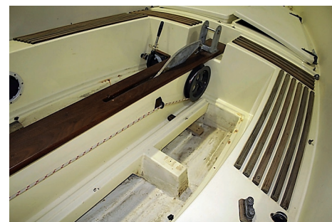
A Norfolk Oyster stripped for maintenance. Note the positively massive sub-frame bonded to the outer hull and reinforcing the centreplate box.
